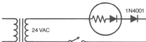
FIGURE 3: AC OPERATION FROM 24 VAC
